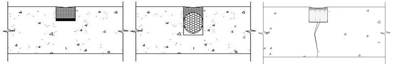
2. The backer rod supports tooling so after installation of material the sealant can be pushed to the bond line with a spatula, ensuring wet-out of the sealant to the substrate.
